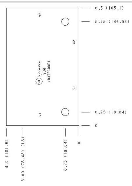
Cartridge extension measurement is to the centerline of the cartridge.
