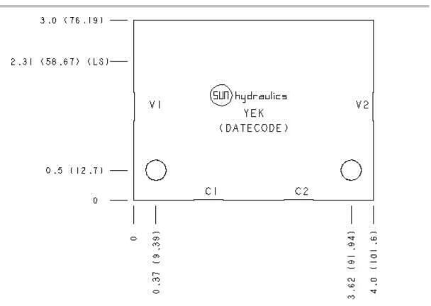
Cartridge extension measurement is to the centerline of the cartridge.
