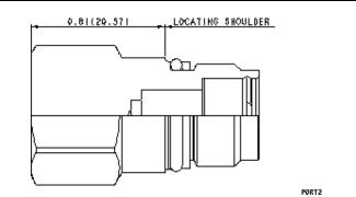
This cavity plug allows all ports to remain open.
