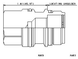
This cavity plug allows ports 1 and 2 to remain open and blocks port 3.
