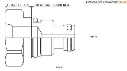
This cavity plug includes an external port open to port 1 and blocks port 2.
