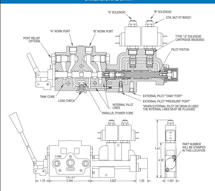
TYPE "-S" SEAL KIT 660580005 SOLENOID CARTRIDGES SEAL KIT 660590008
