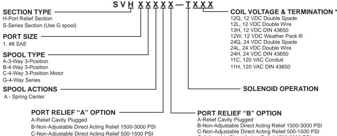
B-Non-Adjustable Direct Acting Relief 1500-3000 PSI C-Non-Adjustable Direct Acting Relief 500-1500 PSI G-Adjustable Direct Acting Relief 1500-3000 PSI H-Adjustable Direct Acting Relief 500-1500 PSI
