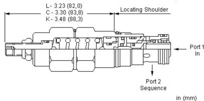
Atmospherically referenced, direct-acting sequence valves with reverse-flow check will supply a secondary circuit with flow once the pressure at the inlet (port 1) has exceeded the valve setting. Additionally, these valves incorporate an integral check valve to provide reverse flow from port 2 (sequence) to port 1 (inlet). The pressure setting of this sequence valve controls the pressure at port 1 relative to the atmospheric vent.
