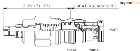
Pilot-operated, balanced poppet sequence valves will supply a secondary circuit with flow once the pressure at the inlet (port 1) has exceeded the valve setting. The pressure setting of a sequence valve controls the pressure at port 1 relative to the pressure at the drain (port 3). These valves are insensitive to back pressure at port 2 (sequence), up to the valve setting. They may be used to regulate pressure in place of 2-port relief valves if there is pressure in the return line.
