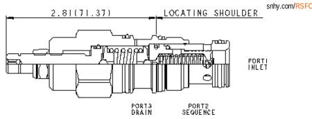
Pilot-operated, balanced piston sequence valves will supply a secondary circuit with flow once the pressure at the inlet (port 1) has exceeded the valve setting. The pressure setting of a sequence valve controls the pressure at port 1 relative to the pressure at the drain (port 3). These valves are insensitive to back pressure at port 2 (sequence), up to the valve setting. They may be used to regulate pressure in place of 2-port relief valves if there is pressure in the return line.
