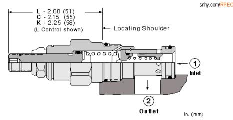
Pilot-operated, balanced-piston relief cartridges are normally closed pressure regulating valves. When the pressure at the inlet (port 1) reaches the valve setting, the valve starts to open to tank (port 2), throttling flow to regulate the pressure. These valves are accurate, have low pressure rise vs. flow, they are smooth and quiet, and are moderately fast.
