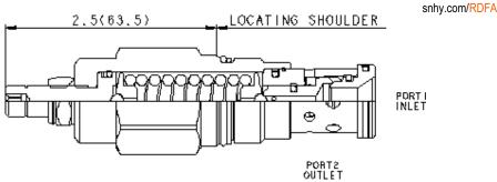
Direct-acting relief cartridges are normally closed, pressure-limiting valves used to protect hydraulic components from pressure transients. When the pressure at the inlet (port 1) reaches the valve setting, the valve starts to open to tank (port 2), throttling flow to limit the pressure rise. These valves are smooth and quiet, essentially zero leak, dirt tolerant, immune to silting and are very fast.
