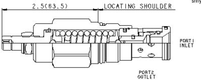
Direct-acting relief cartridges are normally closed, pressure-limiting valves used to protect hydraulic components from pressure transients. When the pressure at the inlet (port 1) reaches the valve setting, the valve starts to open to tank (port 2), throttling flow to limit the pressure rise. These valves are smooth and quiet, essentially zero leak, dirt tolerant, immune to silting and are very fast.
