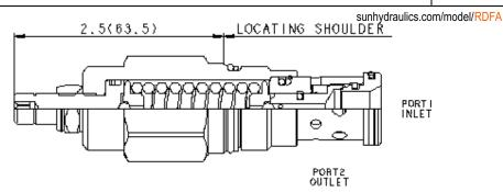
Direct-acting relief cartridges are normally closed, pressure-limiting valves used to protect hydraulic components from pressure transients. When the pressure at the inlet (port 1) reaches the valve setting, the valve starts to open to tank (port 2), throttling flow to limit the pressure rise. These valves are smooth and quiet, essentially zero leak, dirt tolerant, immune to silting and are very fast.
