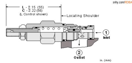
Direct-acting relief cartridges are normally closed, pressure-limiting valves used to protect hydraulic components from pressure transients. When the pressure at the inlet (port 1) reaches the valve setting, the valve starts to open to tank (port 2), throttling flow to limit the pressure rise. These valves are smooth and quiet, essentially zero leak, dirt tolerant, immune to silting and are very fast.
