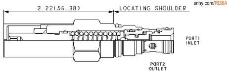
Direct-acting relief cartridges are normally closed, pressure-limiting valves used to protect hydraulic components from pressure transients. When the pressure at the inlet (port 1) reaches the valve setting, the valve starts to open to tank (port 2), throttling flow to limit the pressure rise. These valves are smooth and quiet, essentially zero leak, dirt tolerant, immune to silting and are very fast.
