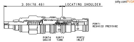
Externally drained, pilot-operated pressure reducing/relieving valves reduce a high primary pressure at the inlet (port 2) to a constant reduced pressure at port 1, with a full-flow relief function from port 1 to tank (port 3). Draining the pilot section at port 4 makes these valves insensitive to pressure at tank (port 3) and provides a means for remote control by pilot or 2-way valves.
