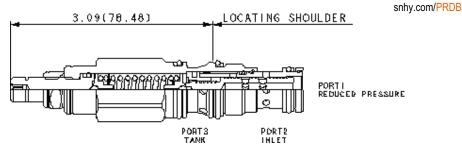
Direct-acting, pressure reducing/relieving valves reduce a high primary pressure at the inlet (port 2) to a constant reduced pressure at port 1, with a full-flow relief function from port 1 to tank (port 3). These valves incorporate a damped construction for stable operation allowing the use of high reduced pressure.
