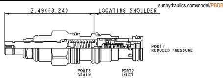
Pilot-operated, pressure reducing valves reduce a high primary pressure at the inlet (port 2) to a constant reduced pressure at port 1, allowing circuits with multiple pressure requirements to be operated using a single pump.
