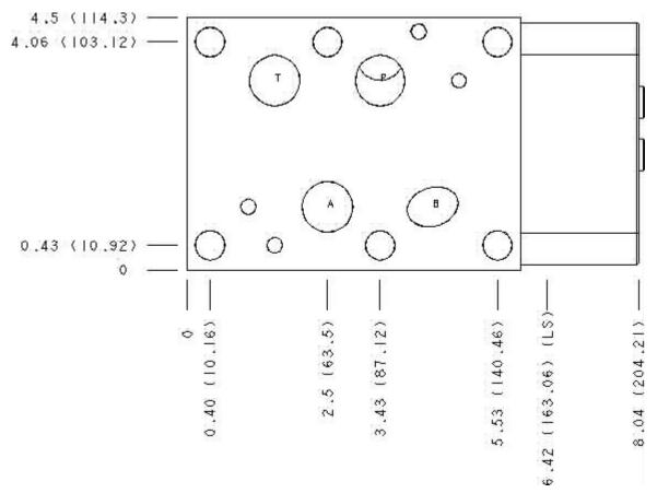
Cartridge extension measurement is to the centerline of the cartridge.
