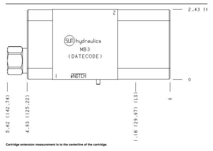
Aluminum Body Pressure Rating: **3000 psi (210 bar)** Ductile Iron Body Pressure Rating: **5000 psi (350 bar)**
