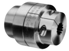
The Clamp-Type Coupling utilizes the basic Magnaloy coupling with the addition of the clamp feature. Developed to compensate for variations in spline formation methods and tolerances. Assures centering of the coupling and positive retention on the shaft. The clamp feature is suggested for all splined couplings, but is also available in smooth bored and keyed models.
