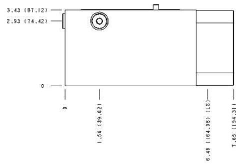
Cartridge extension measurement is to the centerline of the cartridge.
