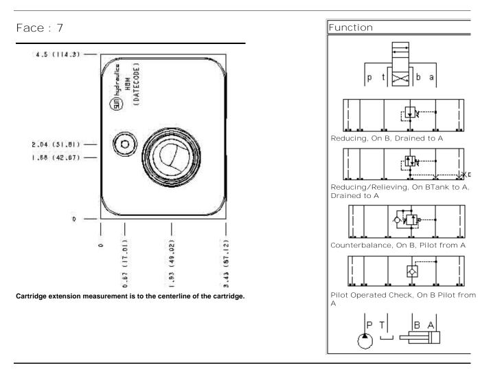
Aluminum Body Pressure Rating: **3000 psi (210 bar)** Ductile Iron Body Pressure Rating: **5000 psi (350 bar)**
