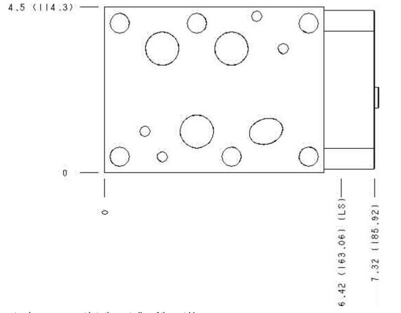
Cartridge extension measurement is to the centerline of the cartridge.
