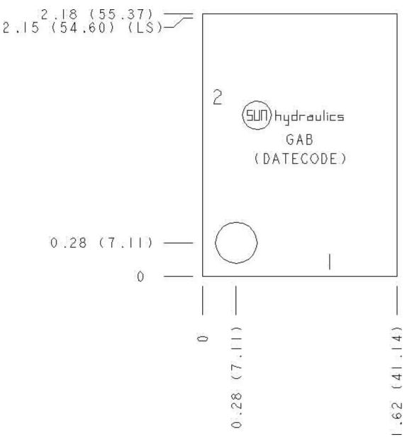
Cartridge extension measurement is to the centerline of the cartridge.
