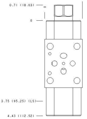
Cartridge extension measurement is to the centerline of the cartridge.
