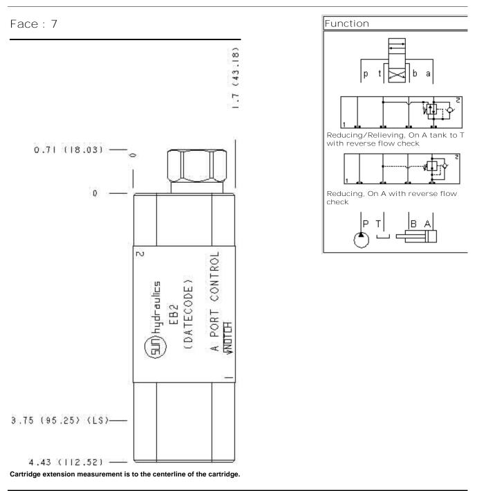
Aluminum Body Pressure Rating: **3000 psi (210 bar)** Ductile Iron Body Pressure Rating: **5000 psi (350 bar)**
