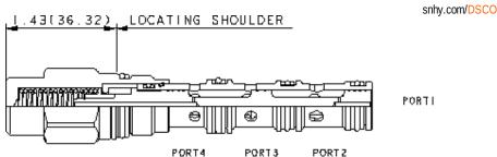
Spring-offset, high-side shuttle cartridges are 2-position valves that have a normal (offset) position that connects the common port (port 3) to work port 4, with work port 2 blocked. When the pressure at port 2 rises above the pressure at port 4, the cartridge shifts to connect the common port to port 2 with port 4 then blocked.
