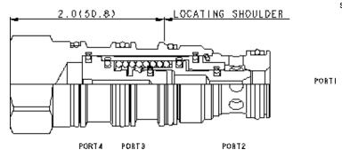
This is a normally closed, balanced poppet, switching element. Pilot pressure at port 3 shifts the valve to the open position.
