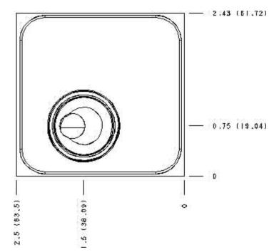
Cartridge extension measurement is to the centerline of the cartridge.
