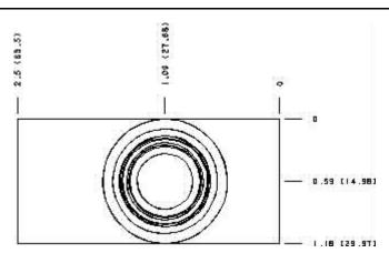
Cartridge extension measurement is to the centerline of the cartridge.
