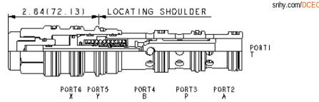
Three-position, 4-way directional cartridges are spring-centered, 6-port directional valves that can be configured from a choice of spool options. The supply port is port 3 and all ports will accept 5000 psi (350 bar). Capacity for these pilot-to-shift valves is dependent on the spool type specified.
