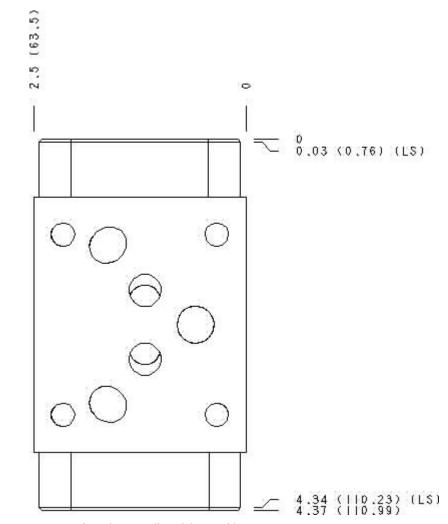
Cartridge extension measurement is to the centerline of the cartridge.
