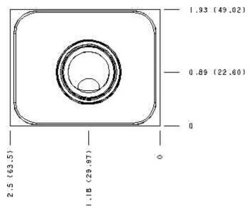
Cartridge extension measurement is to the centerline of the cartridge.
