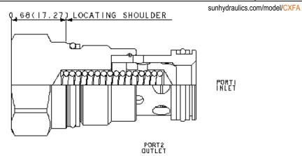
Free-flow, nose-to-side check valves are on/off circuit components that allow free flow from the inlet (port 1) to the outlet (port 2) and block flow in the opposite direction.
