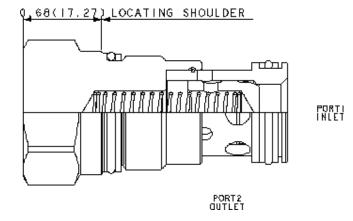
Free-flow, nose-to-side check valves are on/off circuit components that allow free flow from the inlet (port 1) to the outlet (port 2) and block flow in the opposite direction.
