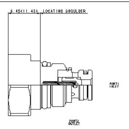
Free-flow, nose-to-side check valves are on/off circuit components that allow free flow from the inlet (port 1) to the outlet (port 2) and block flow in the opposite direction.
