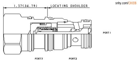
This valve is a pilot to open check valve. It has a non-sealed pilot, a steel seat, and is non-vented. It allows free flow from the valve (port 2) to the load (port 1) and blocks flow in the opposite direction. Pressure at the pilot (port 3) will open the valve from port 1 to port 2. Pilot pressure needed at port 3 to open the valve is directly proportional to the load pressure at port 1. Pressure at port 2 directly opposes pilot pressure.
