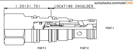
This valve is a pilot to open check valve. It has a sealed pilot, a steel seat, and is non-vented. It allows free flow from the valve (port 2) to the load (port 1) and blocks flow in the opposite direction. Pressure at the pilot (port 3) will open the valve from port 1 to port 2. Pilot pressure needed at port 3 to open the valve is directly proportional to the load pressure at port 1. Pressure at port 2 directly opposes pilot pressure.
