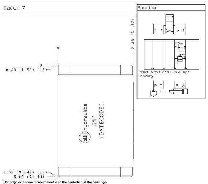
Aluminum Body Pressure Rating: **3000 psi (210 bar)** Ductile Iron Body Pressure Rating: **5000 psi (350 bar)**
