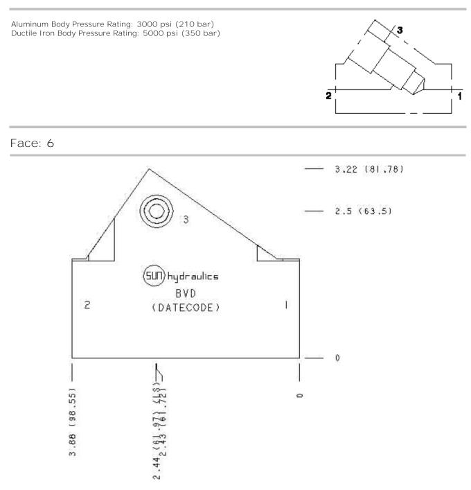
Cartridge extension measurement is to the centerline of the cartridge.
