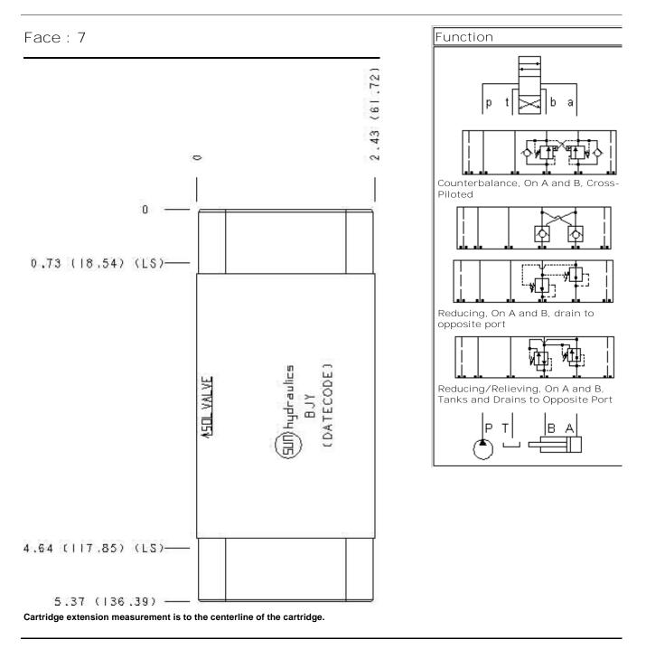
Aluminum Body Pressure Rating: **3000 psi (210 bar)** Ductile Iron Body Pressure Rating: **5000 psi (350 bar)**
