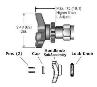
Sun now offers its latest in hand knob control. This ergonomically designed, tri-grip handknob incorporates dual functionality in one package. It can be used to achieve full range control (five turns) or can be used to limit the maximum allowable setting.
