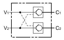
Adaptor Torque CAD 10 = 180 lbf. In.(20.3 N.m) CAD 25 = 480 lbf. In.(54.2 N.m) CAD 50 = 750 lbf. In.(85.0 N.m)
