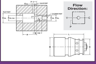
\*Dimensions shown are for NPTF ported valves; for other end fitting configurations consult factory.
