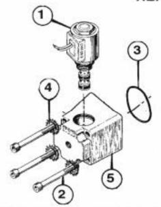
This selector option is not field convertible because a special valve spool is required and spools are matched to the individual bodies. Parts shown are for replacement only. For spring return parts see items 4, 7 and 8 above. Selectors may be ordered with the solenoid option and spring return. For full specifications request Form No. VSOS, VSD and VVS.
