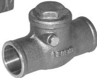
**LEGEND MODELS T-451/S-451** check valves are constructed of heavy duty brass. They have a screwed cap, swing type disc and integral seat. They prevent backflow while offering full flow performance with a minimum of turbulence or pressure loss. Recommended for residential and commercial applications.
