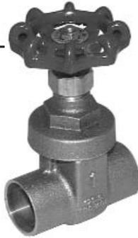
**LEGEND MODEL T-414/S-414** gate valves are constructed of heavy duty bronze. They have a screw-over bonnet, non-rising stem, solid wedge disc and integral seats. The disc is fully guided on both sides for precise alignment. Recommended for commercial and industrial use on steam, water, oil or gas. May be repacked while in service under pressure.
