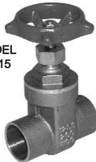
**LEGEND MODELS T-415/S-415** bronze gate valves have a screwed bonnet, non-rising stem, solid wedge disc, and integral seats. The body, bonnet, and disc are manufactured from heavy duty bronze. The aluminum hand wheel has an easy grip configuration. Each valve is tested twice: air under water, in the open and closed position. Recommended for commercial and industrial use on steam, water, oil or gas. May be repacked while in service under pressure.
